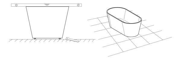
5. Put water in the tub and leave it for few hours to detect any leakage.
